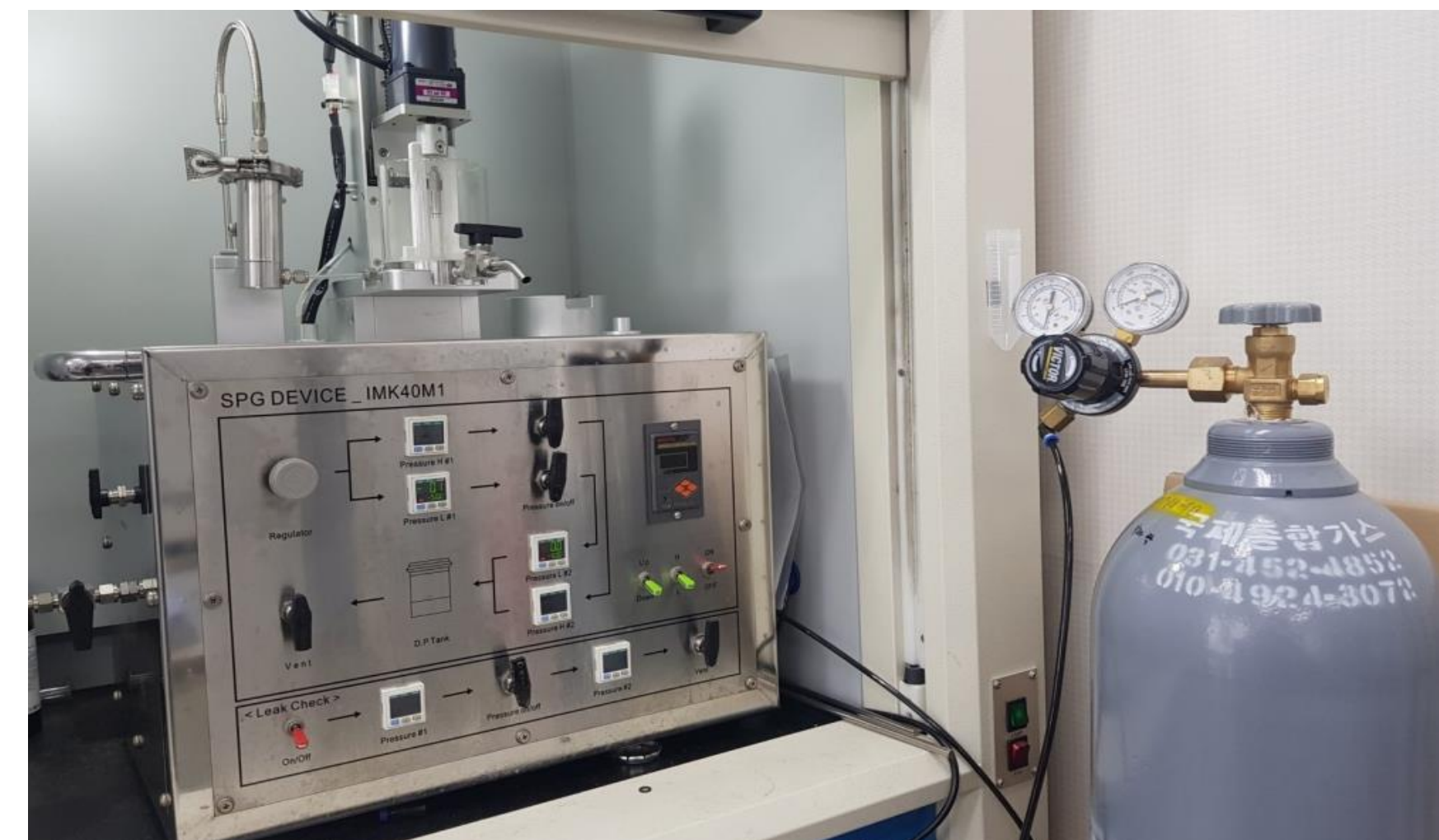
SPG membrane equipment (McTech) for preparing MS which produces uniform size of MS with easy quality control
